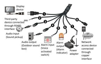
1: Local video output interface (outputting composite video signals), BNC connector
